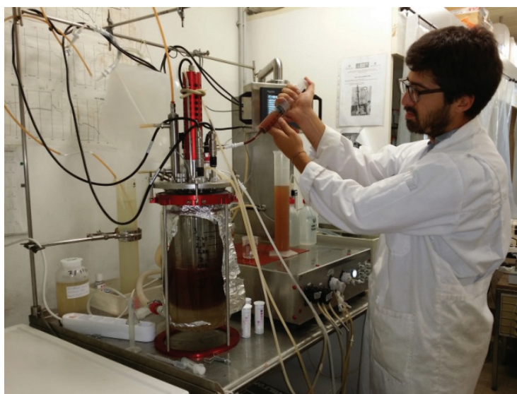
Figure 2.4.15 Execution of batch activity tests. Note the characteristic reddish colour of the enriched anammox culture (photo: Lotti, 2015).
