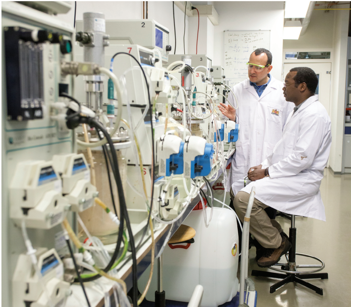
Figure 2.1.1 Experimental facilities for activated sludge activity tests at UNESCO-IHE Institute for Water Education in the Netherlands (photo: UNESCO-IHE).
